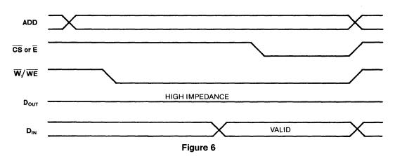
controlled WRITE cycle could be used. This would keep the data-out drivers of the IMS1420's in the high impedance state during the WRITE cycle, preventing any data bus contention with input data.
