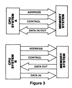
common I/O data bus, while System B has separate data-in and data-out busses.
