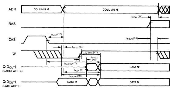
If Column Address N = Column Address M, Cycle is Write-Verify.
