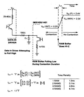
Using:  $C_{I/O}$  (RAM) = 7pF & C (Board)/RAM = 2pF,  $C_T$  = 9pF /RAM
