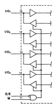
Figure 2: IMS1420/1421 I/O Buffer Enable Conditions
