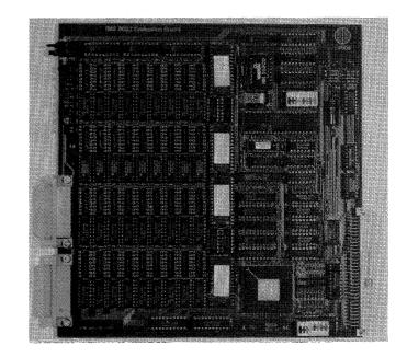
The IMS B002 evaluation board enables users to evaluate and demonstrate the use of transputers. The board is one of a family of compatible evaluation boards. It provides standard buffered INMOS link connections and external control of the transputer's Reset and Analyse functions. This allows it to control a subsystem consisting of other compatible boards, or to be a component of such a subsystem.
