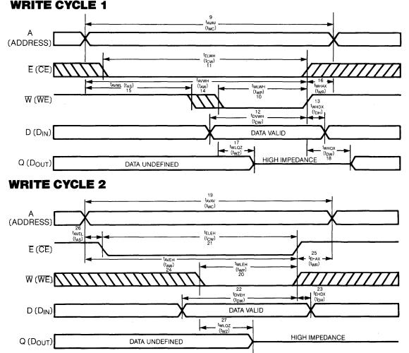
CYCLE 1. Chip Enable access time is not affected by the duration of the deselect interval.
