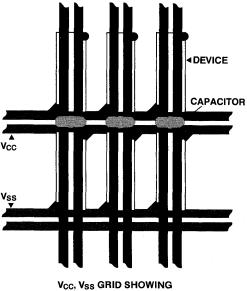
VCC, VSS GRID SHOWING DECOUPLING CAPACITORS
