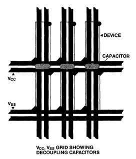
devices in the array (see drawing). A larger tantalum capacitor with a value between  $22\mu$ F and  $47\mu$ F should be placed near the memory board edge connection where the power traces meet the backplane power distribution system. These larger capacitors provide bulk energy storage to prevent voltage drop due to the main supply being located off the memory board and at the end of a long inductive path.
