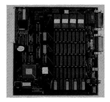
The IMS B001 evaluation board enables users to evaluate and demonstrate the use of transputers. The board is the first of a family of compatible evaluation boards. It provides standard buffered INMOS link connections and external control of the transputer's Reset and Analyse functions. This allows it to control a subsystem consisting of other compatible boards, or to be a component of such a subsystem.
