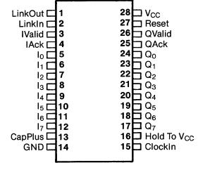
The C001 is available in a 600 mil 28 pin DIP package.
