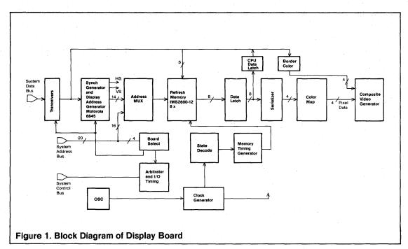
cursor, reverse character video, and blinking. Also, the circuitry to generate a vertical interval interrupt is included to facilitate updating on the screen in such a way as to eliminate the hashing of the display that would occur if screen updates were made during the scan interval.
