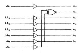
Figure 2: IMS1400 Address Encoder Circuit
