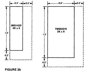
The 4K x 4 is 0.3 square inches while the 2K x 8 is 0.72 square inches. When mounted on a printed circuit board, there must be room added for spacing purposes (assume 0.2" per side). Thus, the effective space required for each device is shown in Figure 2b. The 4K x 4 requires only 0.6 square inches, while the 2K x 8 needs 1.12 square inches.
