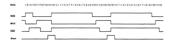
Figure 2b. CPU Access or Retrace Interval Memory Timing
