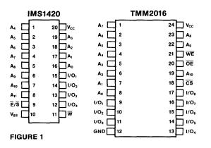
The new 2K x 8 static RAMs have definite applications in microprocessor systems where small amounts of RAMs are required. When the total amount of RAM exceeds 2K bytes, however, the 4K x 4 static RAM becomes a cost-effective alternative.
