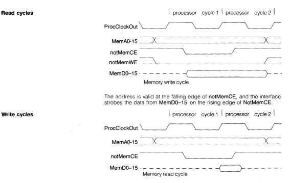
The signal **notMemWE** is held low before the beginning of the cycle. The address is valid at the falling edge of **notMemCE**. The interface presents the data on **MemD0–15**, which is strobed on the rising edge of **notMemCE**.
