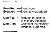
An interrupt request from a peripheral may be signalled via the **EventReq** pin, which is handshaken using **EventAck**. This will normally be used to trigger a high priority process. The request appears to the process as an input on a hardware channel.
