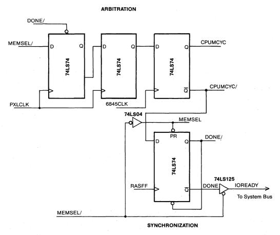
Figure 6. Arbitration and Synchronization
