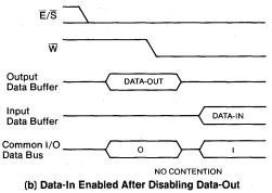
data-in is still enabled (See Figure 5a). Contention can also exist if  $\overline{W}$  goes high (inactive),  $\overline{E/S}$  remains low (active), addresses remain stable, and data-in changes
