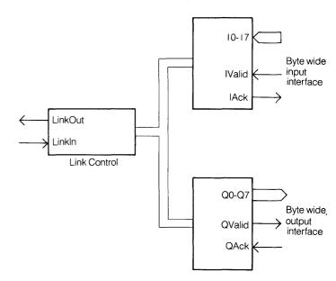
The IMS C001 link adaptor converts between an INMOS serial link and two fully handshaken byte–wide interfaces. One interface is for data coming from the serial link and one for data going to the serial link.
