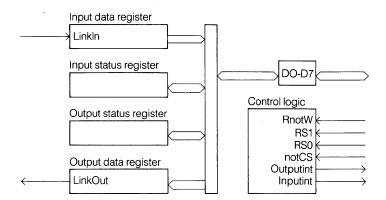
The IMS C002 link adaptor provides an interface between an INMOS serial link and a microprocessor system bus, via an 8-bit bidirectional interface.
